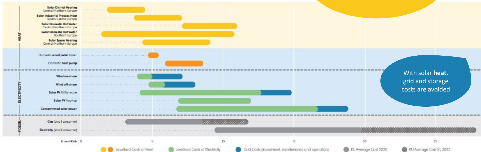
LCOE (Levelised Cost of Energy) € cent per kWh for different Energy Sources
